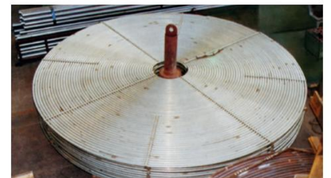
Annealing of various coil pipe systems A wide range of different heating coil systems
