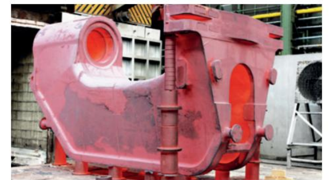
Pearlizing a press stand Isothermal annealing of a press frame
