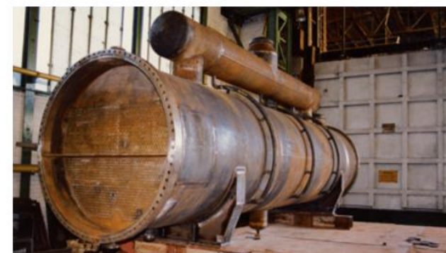
Stress relieving of a heat exchanger Stress-free annealing of a heat exchanger
