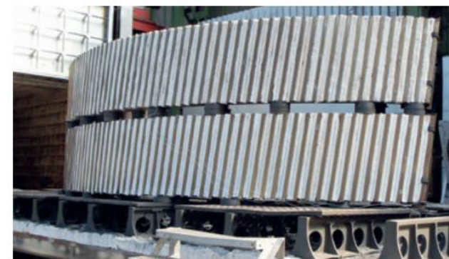
Tempering gear ring segments made of ductile iron Tempering sprocket rim segments made of spheroidal graphite iron
