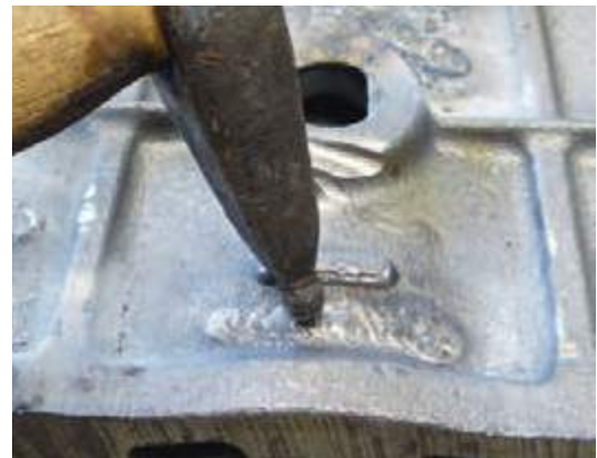
Short stringer bead after slag is removed
