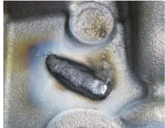
Short stringer bead before slag is removed
