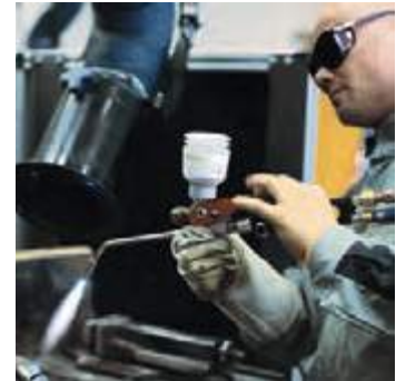
Spray and fuse process from cast repair with UTP SIMmelt™ NiBas25
