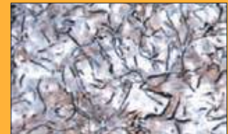
Lamellar Cast Iron Standard (DIN EN 1561): GJL
