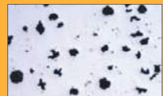
Malleable Cast Iron (graphite flakes) Standard (DIN EN 1562): GJMW / GJMB
