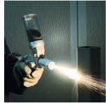
Cold Spray process with UTP COLDmelt™ stainless 18
